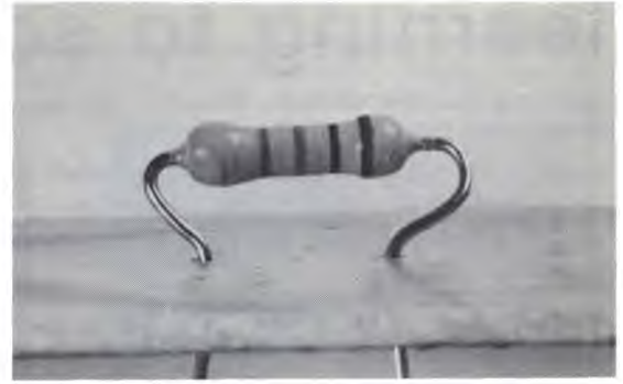
Figure 4: This is an example of a poorly inserted resistor. As the body of the resistor is longer than the hole spacing it would have been advisable to insert as shown in Figure 5.
